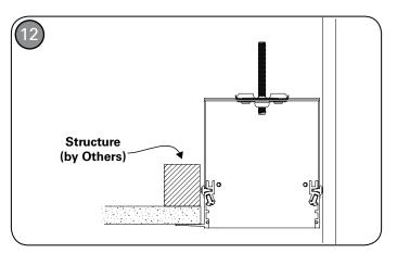
Install blocking (FSR); gypsum board to meet fixture flange as required.
