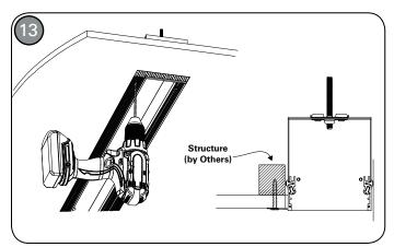
FOR FSR ONLY: Drive screws (provided by others) through fixture flange into structure as shown. Size and length of screws determined by local building code.
