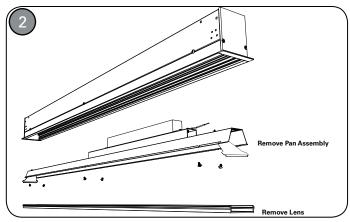
Prior to installing fixture: Remove top access plate. Turn fixture over and remove lens using lens removal tool per lens instruction provided. Remove screws and carefully lift LED tray assembly from housing frame. Disconnect wire-harness quick connects and store pan assembly in a safe place. Lens diffusers do not need to be removed from pan assembly. Repeat for each LEDTray.
