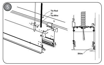
Secure fixture to structure via tie wire or 1/4" tie rod and nut as required. Note: If desired or required, J-rail allows for up to 3/16" adjustment. Fixture can be shimmed for a shadow reveal effect if desired. Standard mounting is flush against wall.
