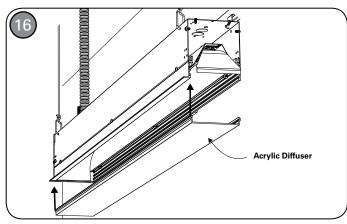
Reinstall acrylic diffuser by squeezing one end, inserting that end into the fixture opening and slowly pressing the diffuser into the housing along the length of the lens until it snaps into place. For continuous runs, ensure seams of adjacent lenses are touching to avoid light leak. Diffuser film should not require re-installation, however, if required, insert tabs into the slots of the LED tray assembly with the shiny side facing toward the LED array.
