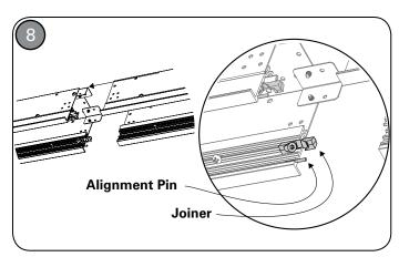
FOR CONTINUOUS ROWS: Repeat step 2 (and 3 for FSR) to prepare fixture. Slide fixtures together ensuring alignment pins are in the correct position.
