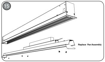
With fixture securely secured in opening, reconnect the first tray assembly to the power feed. Carefully tuck all wiring back into fixture. Reinstall screws to secure tray assembly back into housing. Continue reinstalling additional LED tray assemblies in the same manner using the quick disconnects pre-installed on the LED tray.
