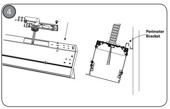
Secure shielded cable to access plate. Reinstall access plate pulling wiring through housing. Lift fixture onto J-rail via perimeter brackets on side of fixture.
