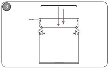
Remove 1/4" knockouts to line up with threaded rods. FOR FSR ONLY: Using (2) 8-32 screws from the LED tray assembly, install aperture guide snugly to ensure housing opening does not open or close during installation. NOTE: This will be removed prior to reinstalling the lens.
