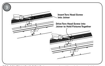
FOR CONTINUOUS ROWS: Insert torx head into joiner and drive screw into housing to hold fixtures together. Ensure there are no gaps between fixtures and joint is secure.
