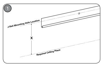
Mark wall at desired location for mounting J-rail. Use dimension "X" as shown on table of page 1 for locating the correct ceiling to mounting hole location. Using J-rail as a template, mark hole locations along wall for pre-drilling where needed. Secure J-rail to wall. Hardware, bracing, and other structural support for J-rail to be supplied and installed by contractor as needed. J-rail hole diameter is 1/4" so #12 screws recommended.
