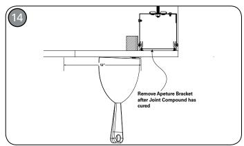
FOR FSR ONLY: Apply a generous amount of joint compound to fixture flange and "feather" at least 12" from fixture aperture. Ensure compound has properly cured before removing aperture bracket.
