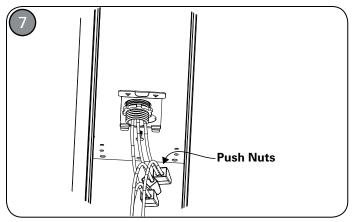
Connect feed wiring to fixture through wiring via push-in quick connects or wire nuts.
