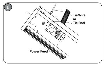
Wiring should enter fixture housing as shown. Ties rods extend into housing and are secured with nuts. Tie wires can be looped through holes in top of housing if used instead of tie rods.
