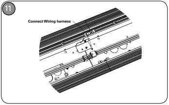
Make appropriate wire connections between fixture housings using provided connectors.
