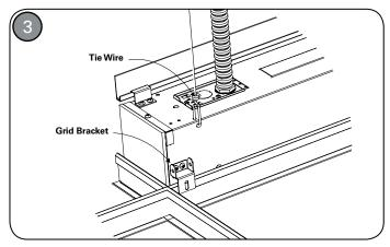
Secure fixture to structure via tie wires as required by local building code. Note: If desired or required, J-rail allows for up to 3/16" adjustment. Fixture can be shimmed for a shadow reveal effect if desired. Standard mounting is flush against wall. OPTIONAL STEP: Secure fixture to grid using #8 screws through grid bracket. Required for seismic installations.
