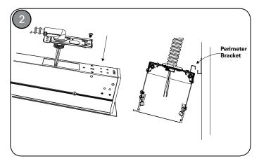
Remove access plate on top of fixture. Secure shielded cable to access plate. Connect power wiring to fixture. Reinstall access plate pushing wiring back through housing. Lift fixture onto J-rail via perimeter brackets on side of fixture.
