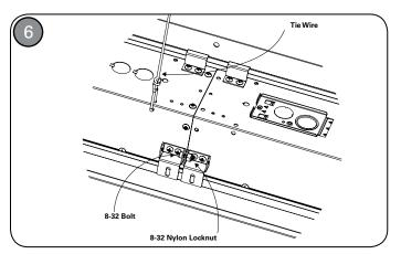
FOR CONTINUOUS RUNS: Secure run using #8-32 bolt and nut. Add tie wire for additional support where required.
