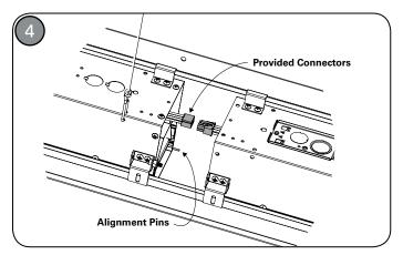
FOR CONTINUOUS RUNS: Hang next fixture in row on J-rail as in step 2. Connect through wiring using the provided push in connectors. Tuck wiring into fixture and push together ensuring alignment pins are properly connected.
