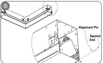
FOR CORNER INSTALLATION: Prepare corner unit for installation. Identify power feed side (end toward Beginning of Run). Prep wires on power feed side for connection to previous section in the run / pattern. Install alignment pins into extrusion non-power feed side using a hammer.Tapered side should face outward.
