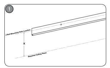
Mark wall at desired location for mounting J-rail. Use dimension "X" as shown on table of page 2 for locating the correct ceiling (bottom of grid) to mounting hole location. Secure J-rail to structure. Hardware, bracing, and other structural support for J-rail to be supplied and installed by contractor as needed. J-rail hole diameter is ¼" - #12 screws recommended.
