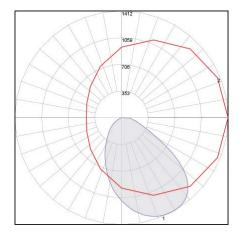
Filename: 23XR-2L35-ETG-4-1DD-SI-W Test Number: P24876 Lumens: 2839 Lm Watts: 37.3 W LPW: 76 Lms/W CCT: 3500K
