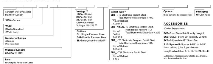
NOTES: <sup>(1)</sup> Products also available in non-US voltages and frequencies for international markets. <sup>(2)</sup> Not available when specifying emergencies, voltage must be specific. <sup>(3)</sup> Stem mounting not available on 3-lamp fixtures. <sup>(4)</sup> 2 point suspension recommended for 2 and 4-lamp fixtures. <sup>(5)</sup> Steel endplates with 7/8" KO standard for continuous row mounting. <sup>(5)</sup> Please specify required voltage, 120V or 277V.
