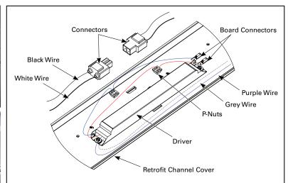
Connect the green ground wire from the gear tray to the ground of the housing. A linear disconnect is provided for simple installation to the existing disconnect (if equipped) or independently connect all of the fixture wires to power supply wires: white to white, black to black and optional blue wire for EM version (not shown). If applicable, connect purple and grey to dimming system.
