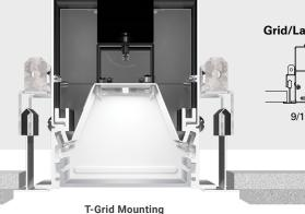
Grid/Lay-in Concealed T Slot Grid
