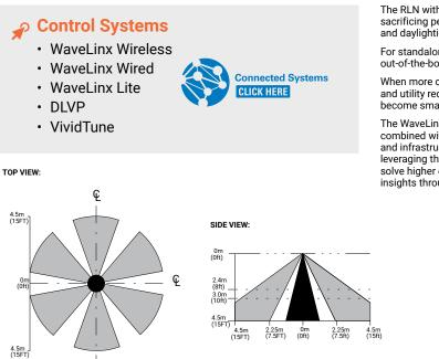
**Note**: Installation of integrated sensors within 3-ft (1m) of HVAC air vents is not recommended. The pattern shown is intended solely as a general guide and is not to scale.
