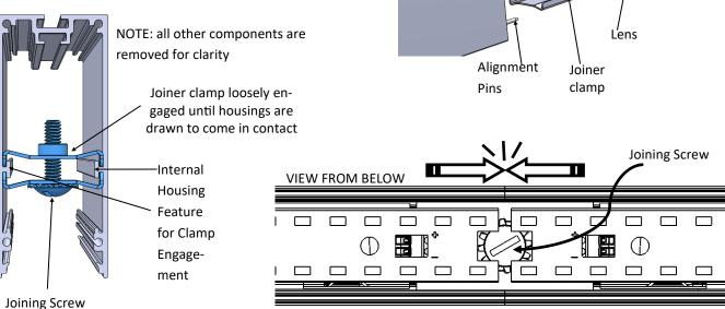
From below, with the lens removed, the joiner bracket screw should be visible and self-centered about the gap between and behind adjacent LED boards. Fasten screws while ensuring that housings are still squarely in contact with each other to complete the joining of each subsequent continuous row fixture. Re-insert lens into its position.
