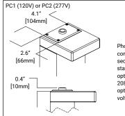
Photocontrol cover is precision machined from corrosion-resistant 6061-T6 aluminum and is secured to bollard head with tamper resistant stainless steel hardware. The photocontrol option is available in dedicated 120V or 208-277V. When specifying a photocontrol option make sure to designate the appropriate voltage within the catalog logic.
