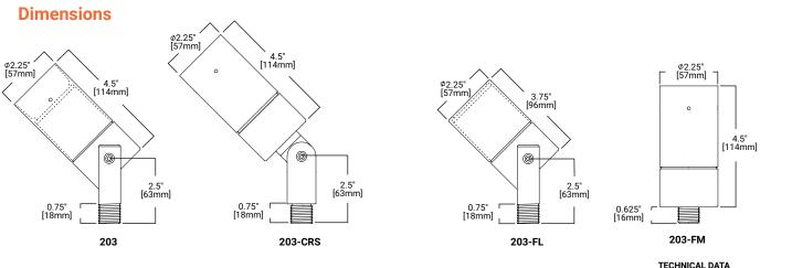
TECHNICAL DATA 8W LED, L70/60,000 hours at 25°C Low Voltage: 50W Halogen MR16
