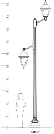
Mounting: CRF-1A Mid pole Luminaire: S2-LE3-CP Mounting: CRFT-F Pole: RTA500-MPL
