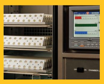
Precision design practices and rigorous reliability testing result in dependable luminaries that thrive in outdoor environments. RL LED Cobrahead is rated for operation in -30°C to 40°C ambient environments [for 50°C ambient, specify HA option], comes equipped with 10kV transient surge protection and is backed by a five-year warranty from a world class manufacturer.
