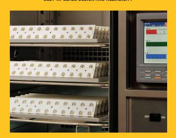
Precision design practices and rigorous reliability testing result in dependable luminaries that thrive in outdoor environments. Ridgeview LED is rated for operation in -30°C to 40°C ambient environments [for 50°C ambient, specify HA option], comes equipped with 10kV transient surge protection and is backed by a five-year warranty from a world class manufacturer.
