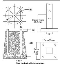
Number of Bolts Template Bolt Num **Bolt Circle Bolt Size** SSS4 TMP1 AR1 85-110 4  $3/4 \times 25 \times 3$ SSS5 TMP1 AB1 11.0 4 3/4 x 25 x 3 SSS6 TMP2 AB3 12.5 4 1 x 36 x 4
