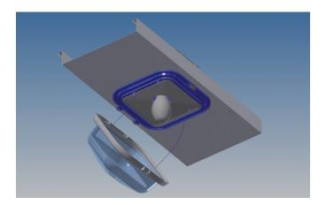
Step 3: Install wiring guide into lamp socket cavity.
