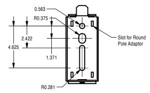
3. Position the Luminaire Bracket, square and straight, up against the luminaire mounting surface. HEX bolt head is always on the PQMH and PQM15 side
