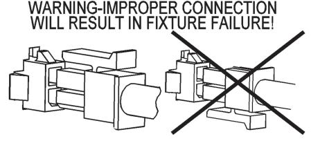
3. LED strips are quick-connected together in the following MAXIMUM lengths:
