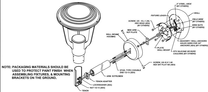
1. SCREW STUDS INTO NUTPLATE. SLIDE WALL MOUNT HOUSING OVER STUDS. SLIDE EXTRUDED ARM & ADAPTER OVER STUDS. INSERT STUDS THRU HOLES IN TENON. INSTALL LOCKWASHERS & HEX NUTS ONTO STUDS AS SHOWN. TIGHTEN NUTS TO 35-40 FT/LBS TORQUE.
