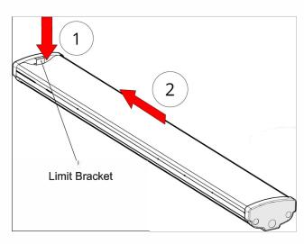
Step 2: Gently press down on one side of the lens approximately 1" to reveal a limit bracket. Slide the lens toward the end being pressed. This will allow the opposite end to become free and lift out.
