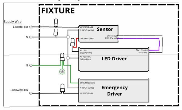
\*\*WARNING: Do not supply AC power to the switched line until AC power is supplied to the unswitched line.
