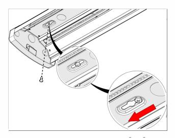
Step 5: Install the mounting hardware in the marked positions, leaving them slightly untightened. Align the keyholes in the fixture with the hardware in the ceiling and slide the fixture until the screws slide into the narrow ends of the keyholes. Tighten the hardware.
