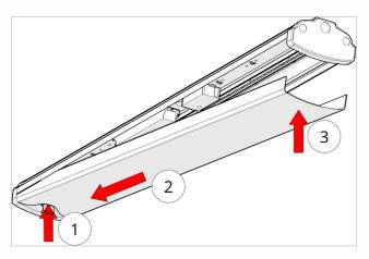
Step 7: Replace the lens by inserting one end of the lens into the end cap with the limit bracket. Press down slightly to keep the top of the lens under the bracket. Fit the opposite end of the lens into the fixture.
