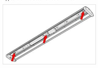
Step 4: Position the fixture in the desired location and mark the center of the keyholes. Remove the appropriate knockout from the fixture.
