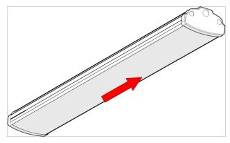
Step 8: Once the lens is fully fitted in the fixture housing, slide the lens towards the opposite end cap to lock the lens in place. Restore power\*\* and check that the fixture is functioning properly.
