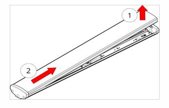
Step 3: Lift the opposite end of the lens and slide the lens out of the fixture. Set the lens aside.
