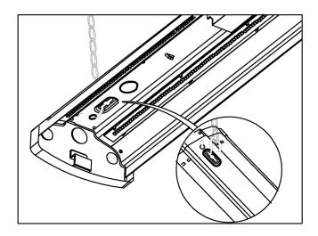
Step 6b: Slide "S" hook into key hole detail and through adjacent hole as shown at each end of fixture.
