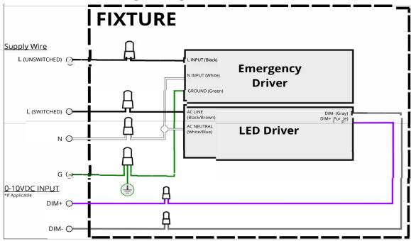
\*\*WARNING: Do not supply AC power to the switched line until AC power is supplied to the unswitched line.
