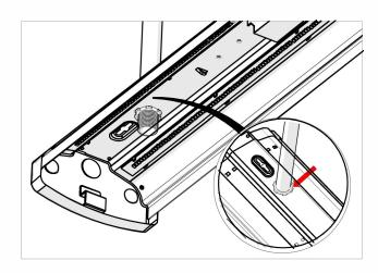
Step 4b: Remove the appropriate knockouts from the fixture. With help from another person, fit the 1/2" conduit\* through the knockouts.
