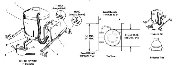
Complete Fixture consists of Reflector Trim & Frame-In Kit. Select each separately.
