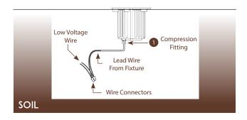
Hand tighten compression fitting 1 (Do not use tools and do not over tighten)
