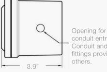
Opening for 1/2" conduit entry. Conduit and conduit fittings provided by
