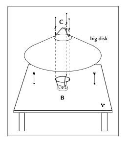
5. Insert element C and tighten the three screws on element B
