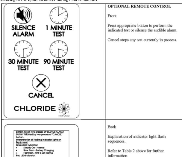
Single Flash - Battery Fault Double Flash - Lamp Failure
