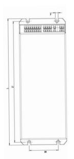
Length (L) typical: 230 mm / 9.06 in Width (W) typical: 80 mm / 3.15 in Height (H) typical: 30 mm/1.18 in
