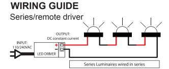
Diagrams are a guide only, wire colours and polarity may change depending on fixture and country
