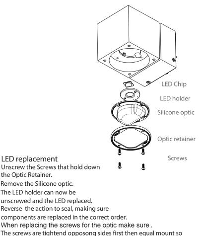
There is equal pressure on the optic retainer
