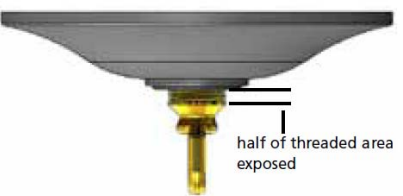
Drawing 2 – Canopy Adjustment
