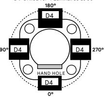
D2@90 Drilled for 2 Luminaires at 90°
