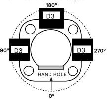
D4 Drilled for 4 Luminaires at 90°
