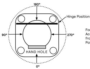
For Factory Installed Options and Accessories, Specify Orientation from Hand Hole and Height Above Pole Base Where Required.
