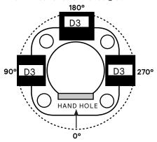
D4 Drilled for 4 Luminaires at 90°
