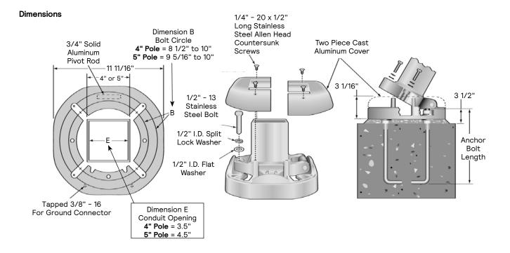
NOTE: Factory supplied template must be used when setting anchor bolts. Gardco will not honor any claim for incorrect anchorage placement from failure to use factory supplied templates.
