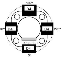
D2@90 Drilled for 2 Luminaires at 90°
