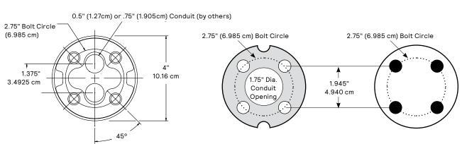
**NOTE**: Factory supplied template must be used when setting anchor bolts. Gardco will not honor any claim for incorrect anchorage placement from failure to use factory supplied templates.
