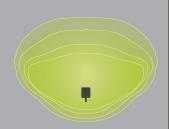
5' Setback, 25° Tilt 50% Main Beam: 81°H x 39°V 10% Field Beam: 119°H x 77°V
