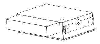
**Step 1 - Grid Ceiling Mount (14-1/4" x 9-1/8"cutout required)** Note: This product is U.L. approved for use in IC rated ceiling constructions.
