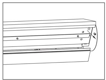
3. Flip the module board. Press one side of the module board to flip the module board to the appropriate position.
