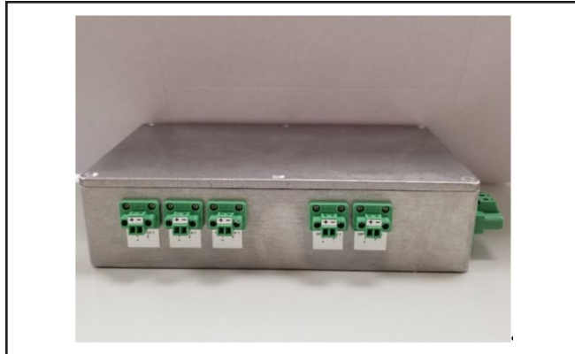
Figure 13. Input terminal connections for the MRI-R6DNLT Distribution Box
