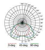
24GTR-4GUV4-R1 Electronic Driver 4 GUV Sources Spacing criterion: (II) 1.34 x mounting height,  $(\bot)$  1.88 x mounting height Irradiance (mW): 28406 Input Watts: 127W Test Report: 24GTR-4GUV4-R1.IES
