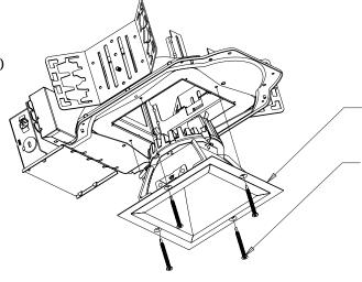
Antimicrobial powder coated security plate attached to the reflector flange with mechanical tabs and high strength adhesive.
