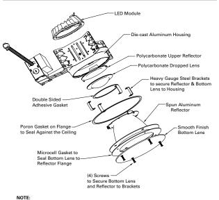
Sealed Medical Regress Lens has gasket on flange to seal against ceiling and is attached to housing with torsion springs.
