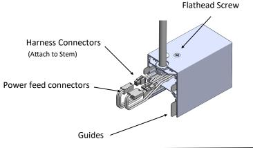
For row mounting fixtures attach male end of harness to female end of harness.
