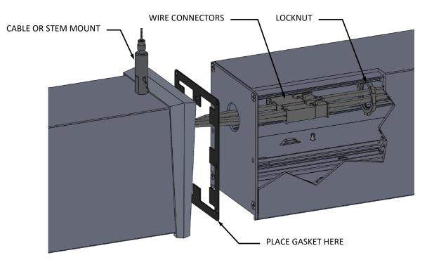
Re-install reflector and lens, being careful not to pinch any wires underneath the reflector.
