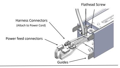
For row mounting fixtures attach male end of harness to female end of harness and slide fixtures together.
