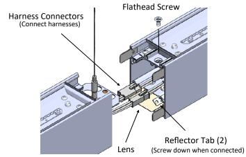
Remove Direct side of fixture to install Endcaps
