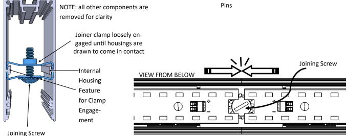
From below, with the lens removed, the joiner bracket screw should be visible and selfcentered about the gap between and behind adjacent LED boards . Fasten screws while ensuring that housings are still squarely in contact with each other to complete the joining of each subsequent continuous row fixture. Re-insert lens into its position.
