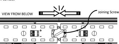
From below, with the lens removed, the joiner bracket screw should be visible and self-centered about the gap between and behind adjacent LED boards. Fasten screws while ensuring that housings are still squarely in contact with each other to complete the joining of each subsequent continuous row fixture. Re-insert lens into its position.
