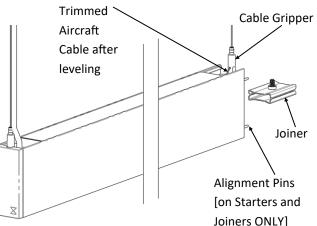
Joiner and Ender fixtures are suspended by one aircraft cable at the far end and depend on the Starter fixture to first be installed.
