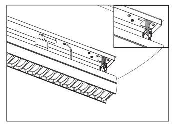
8. Snap fixture onto the surface mount bracket, ensuring that the fixture has fully engaged.
