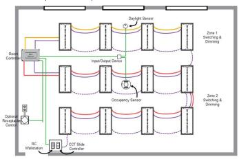
In the sample application, the operation is simplified with the separation of the switching/dimming functions and the CCT control.
