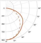
FILE NAME: BRG-WN-3L35-LD2-UNV-22-STD.IES LAMP: (LD2) LED 3500K LUMENS: 2926 Lm WATTS: 28.7 W EFFICACY: 102 Lm/W TEST NO.: P189564 SC: (II) 1.22, (L) 1.30 0° (II) \_\_\_\_\_
