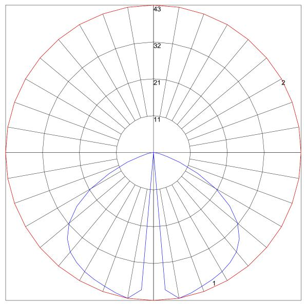
Maximum Candela = 42.74 Located At Horizontal Angle = 0, Vertical Angle = 10 # 1 - Vertical Plane Through Horizontal Angles (0 - 180) (Through Max. Cd.) # 2 - Horizontal Cone Through Vertical Angle (10) (Through Max. Cd.)
