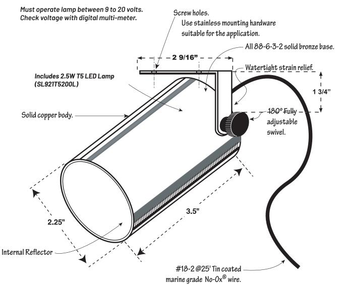
Plan Symbol: Includes 2.5W T5 LED Lamp (SL921T5200L)
