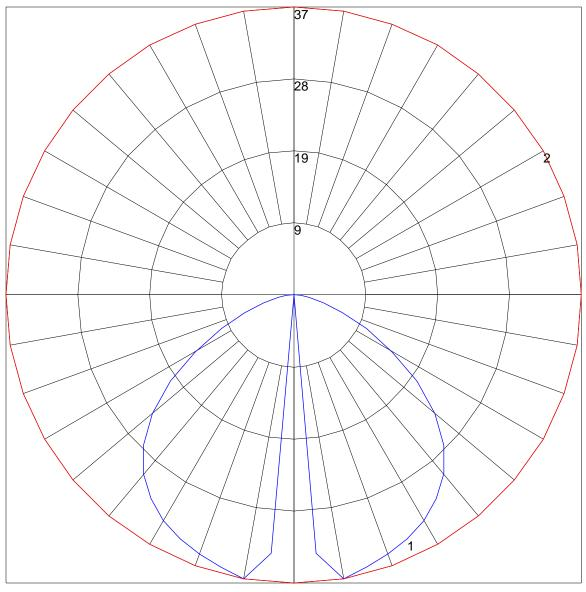
Maximum Candela = 37.45 Located At Horizontal Angle = 0, Vertical Angle = 10 # 1 - Vertical Plane Through Horizontal Angles (0 - 180) (Through Max. Cd.) # 2 - Horizontal Cone Through Vertical Angle (10) (Through Max. Cd.)
