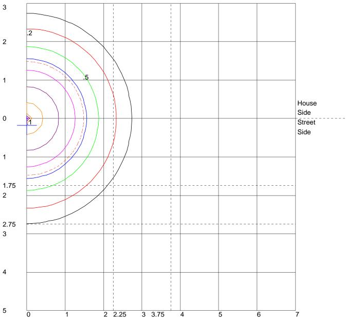
Distance In Units Of Mounting Height Values Based On 1.67 Foot Mounting Height 1/2 Maximum Candela Trace Shown As Dashed Curve
