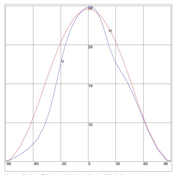
Maximum Candela = 38.2 Located At Horizontal Angle = 0, Vertical Angle = 1
