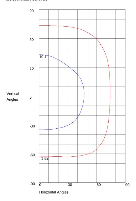
Maximum Candela = 38.2 Located At Horizontal Angle = 0, Vertical Angle = 1 50% Maximum Candela = 19.1 10% Maximum Candela = 3.82
